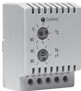
The electronic temperature regulator and humidity controller controls the temperature and humidity level of the air independently of each other by switching resistive and inductive loads (e.g. small heating units and refrigeration units).
