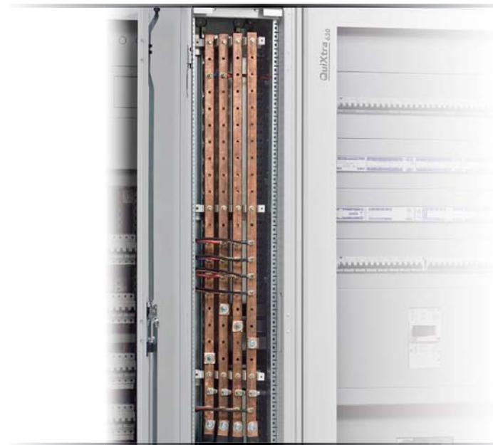
The *staircase busbar* can be installed vertically in the 12 module enclosure and horizontally in the 24 and 36 module enclosures. In either case, functions cannot be mounted on top.
