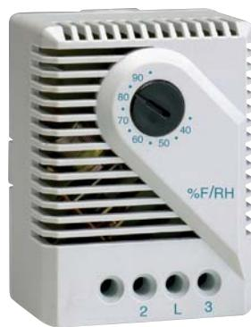
The electromechanical hygrostat is designed to control enclosure heaters so that the dew point is raised when a critical relative humidity of 65% is exceeded.
