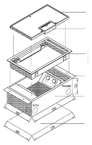
Moulded Polyamide lid with steel insert plate (8mm carpet rebate).
