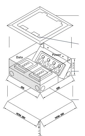
2 x cable exit ports fold down when in use to allow cables to exit with the main cover closed.
