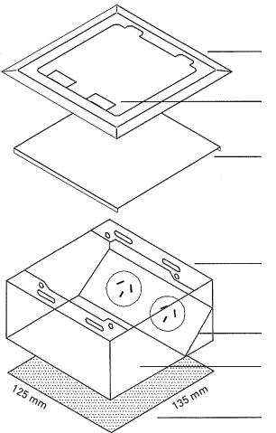
Hinged lid 145 mm x 145 mm, screw fixes to steel box body
