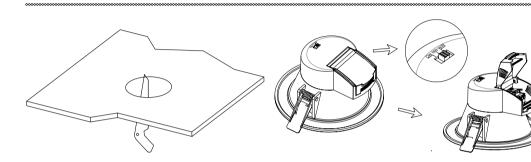
1. Cut a hole in the desired location according to product label
