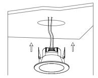
4. Hold back the clips as you push the downlight into the cut hole
