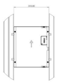
2. Fold out the 4x side tabs of the base box. Insert the base box into the pre-prepared framing. Ensure the arrow is orientated upwards. The side tabs will stop the box at the correct height on the framing to align with standard 10mm wall linings.
