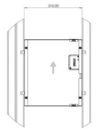
2. Fold out the 4x side tabs of the base box. Insert the base box into the pre-prepared framing. Ensure the arrow is orientated upwards. The side tabs will stop the box at the correct height on the framing to align with standard 10mm wall linings.
