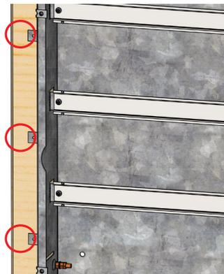
Fold out tabs to sit the board at the right depth in the wall when plasterboard is installed
