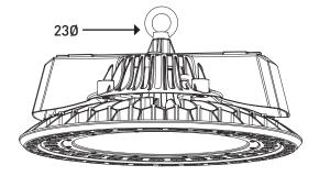
Fix luminaire to a suitable chain/suspension cord (not supplied) for the application.
