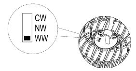
Select the desired colour temperature before installation.
