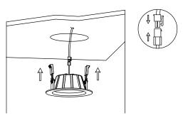
Connect the downlight with driver, hold back the spring clip then push the downlight into the hole.
