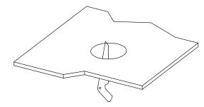
Cut a hole in the ceiling to the cutout size of the LED downlight (see cutout reference table below).
