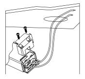
Use a screwdriver to open the driver terminal cover, feed the main AC wire L.N. in terminal block respectively, then fix the cover back on.
